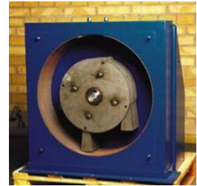
Photo: A 4KSG mounted with a special rotor and hammers.
